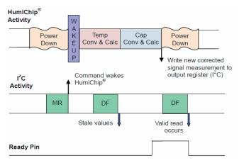
Figure 4.3.3: I<sup>2</sup>C Data Fetching in sleep mode
