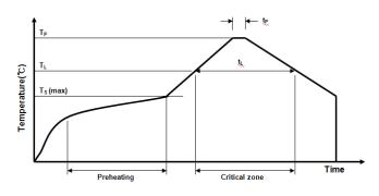
Figure 1.2: Soldering Profile (IPC/JEDEC Standard)  $T_p \le 240 \text{ °C}, t_p < 40 \text{ sec}, T_L < 200 \text{ °C}, t_L < 150 \text{ sec}.$ Ramp-up/down speed < 5 sec
