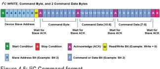
Figure 4.5: I<sup>2</sup>C Command format
