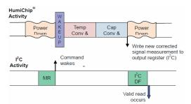
Figure 4.3.2: Measurement sequence in sleep mode
