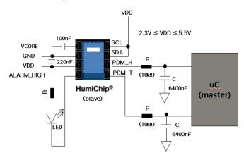
Figure 6.3: LED control with alarm function
