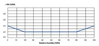
Abbildung 1: Typical RH% Accuracy at 25 °C
