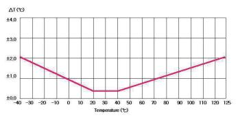
Abbildung 2: Typical Temperature Accuracy
