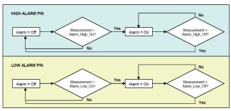
Figure 6.5: Alarm output flow chart
