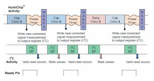
Figure 4.3.1: I<sup>2</sup>C Data Fetching in update mode
